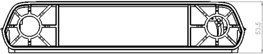
PS3HD Wall Mount Enclosure Dimensions
